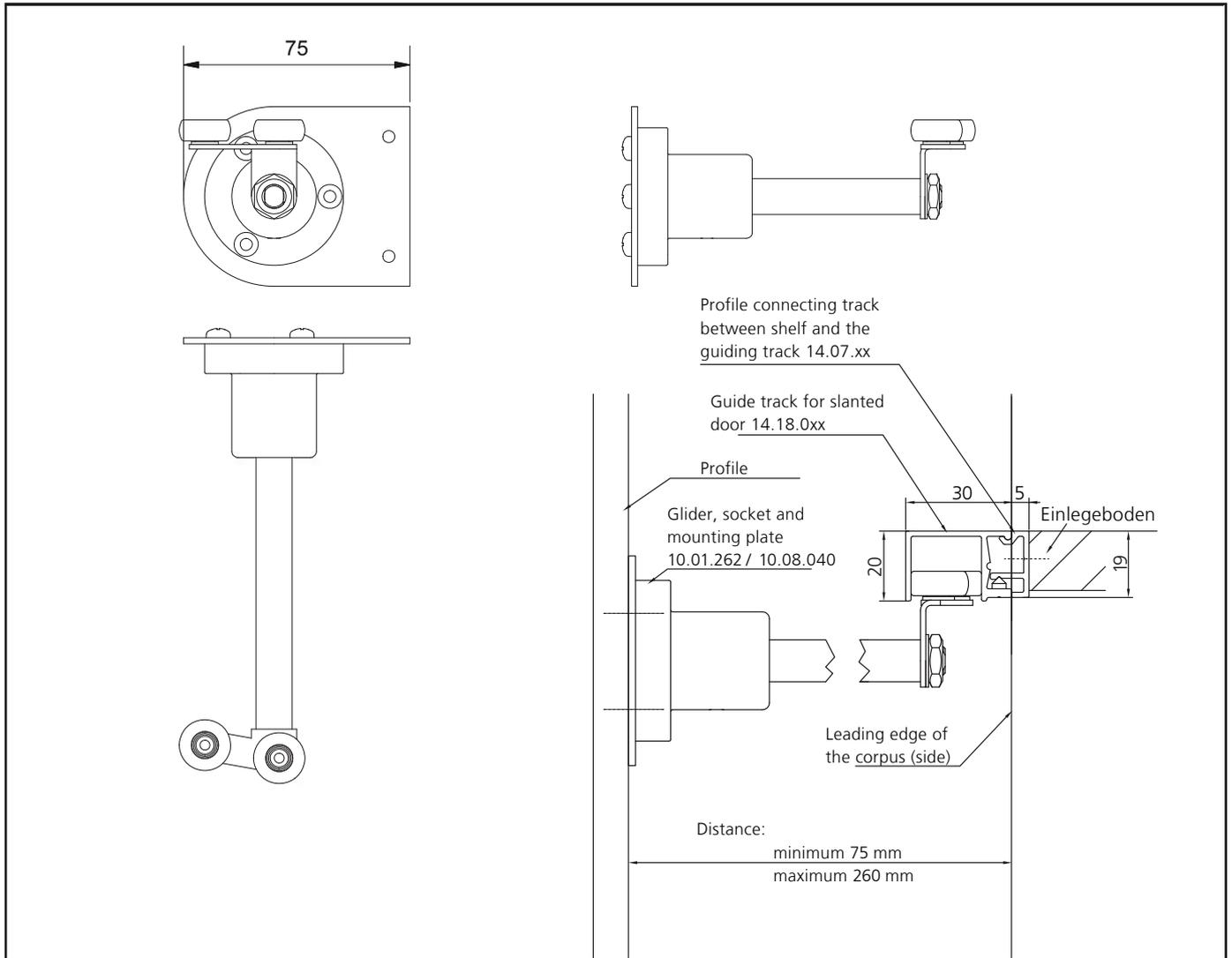
1\_ Installation dimensions of the slanted door guide
